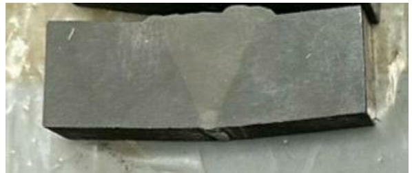
Gambar 26 Makro Material 2 Preheat 50 °C
