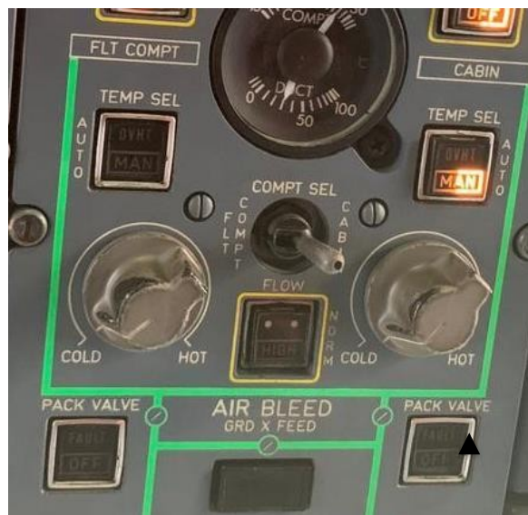
Gambar 5: Overhead panel pack valve normal operation
