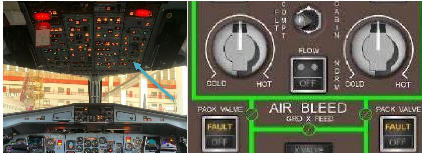
Gambar 3. Fault pack valve on overhead panel
