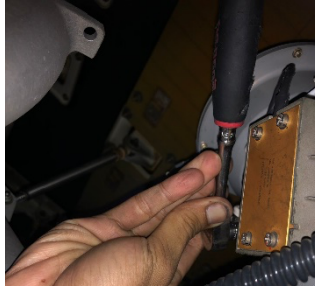
Gambar 6: open coupling Pack valve ATR 72-500/600
