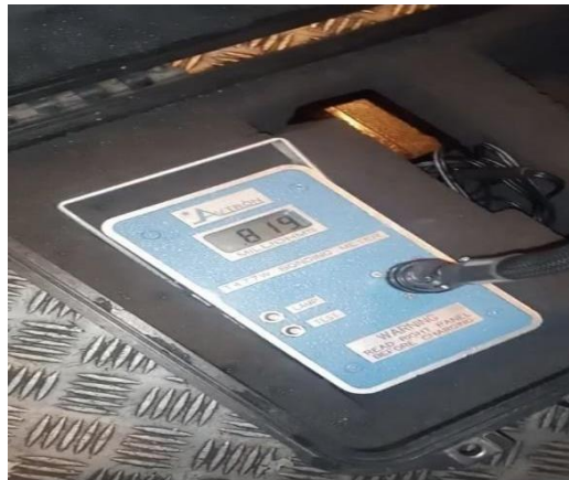
Gambar 8: Evidence measurement of Bonding Lead with bondingmeter
