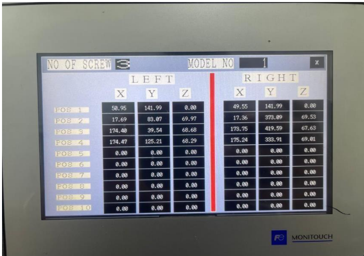
Gambar 62 Display HMI Posisi Screw
