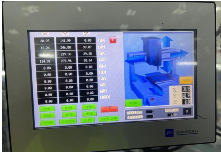
Gambar 64 Display HMI JOG
