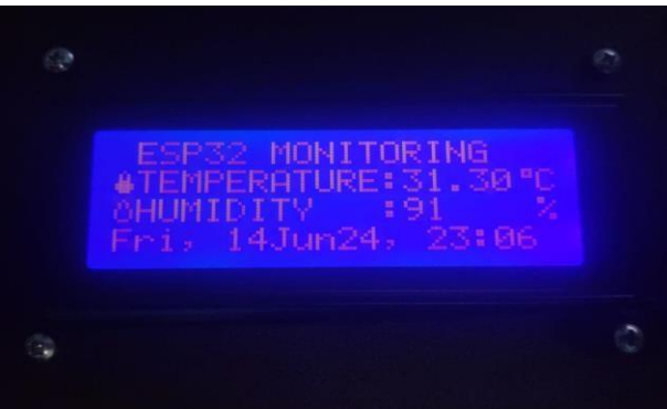
Fig 17. Humidity Out of Limit Display
