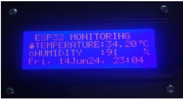
Fig 15. Temperature Out of Limit Display
