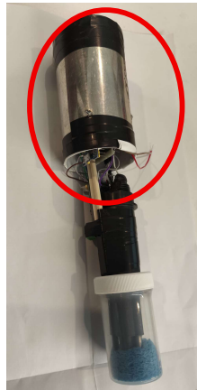
Figure 2.11 Implementation of Faraday Cages on pH Sensors
