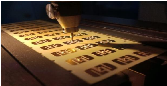
Figure 1. wire bonding process
