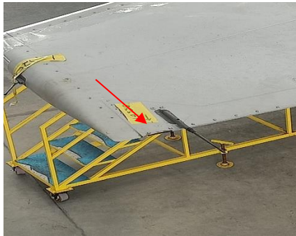
Gambar 6 : Horizontal stabilizer damage
