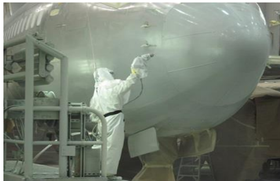
Gambar 2.5 : Top coat finish
