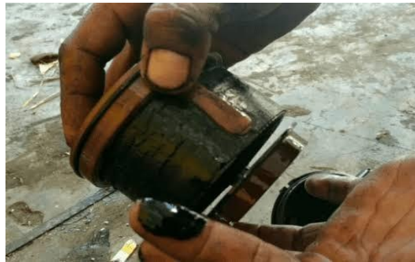
Figure 7. Clogged Fuel Filter After B35 Use
