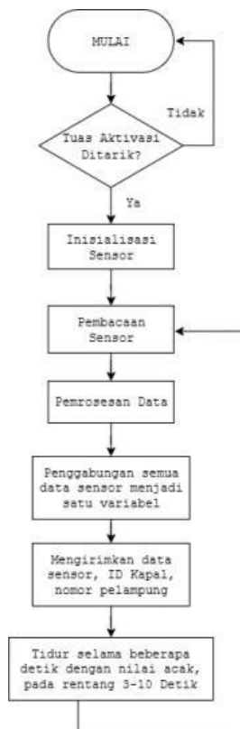
Gambar 19. Flowchart Cara Kerja Sistem Sender ( Transmitter )
