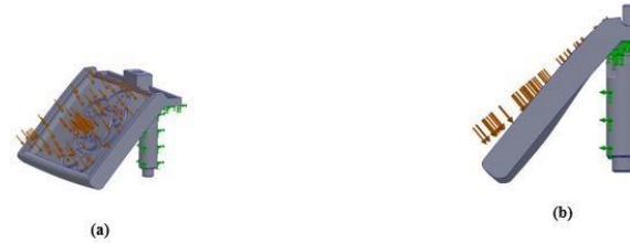
Figure 12. (a) Phone Holder Isometric View (b) Phone Holder Side View. The simulation uses a bonded contact with independent mesh. View (a) shows mesh and constraints; view (b) shows structure under load. This setup confirms the structural stability of the phone holder.
