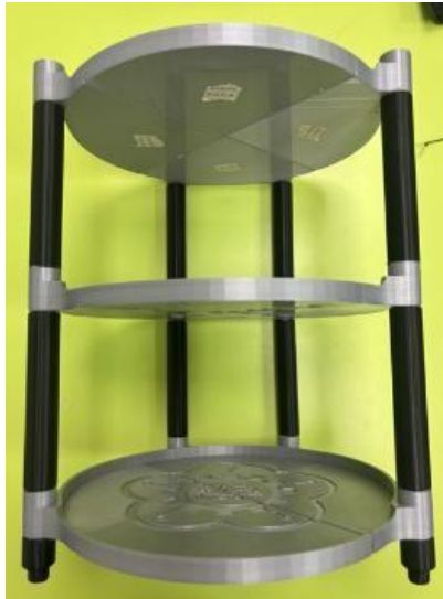
Figure 10. Tray 3D Printing Result Tray 3D Printing Result
