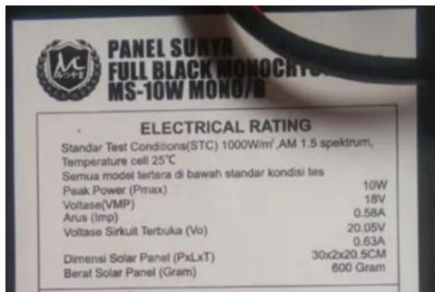
Fig. 8. Solar panel electrical specifications.
