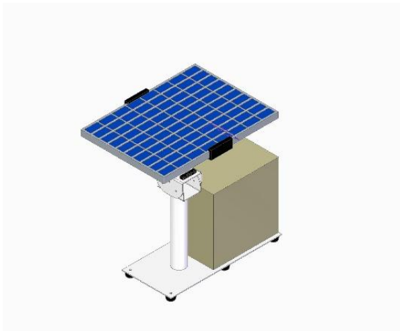
Fig. 4. Mechanical design of the dual-axis mechanism.
