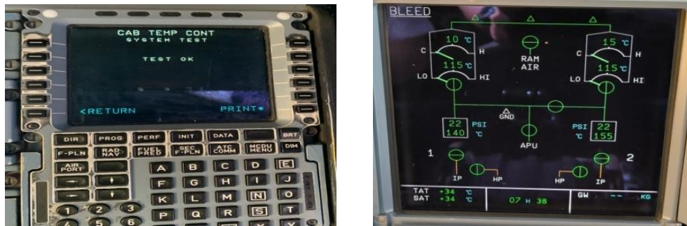
Gambar 6. MCDU dan Indikasi FLOW CONTROL Valve di Cockpit
