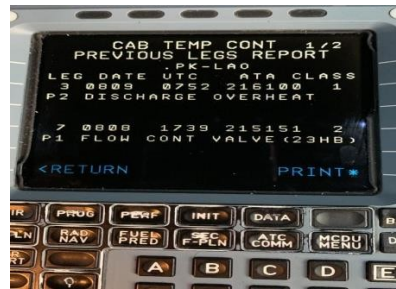
Gambar 3. Hasil Kerusakan Maintenance Message Flow Control Valve 23HB .
