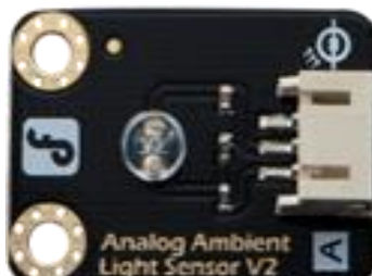
Gambar 2. 4 Analog Ambient Light Sensor V2 [17]
