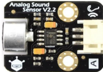
Gambar 2. 3 Analog Sound Sensor [17]
