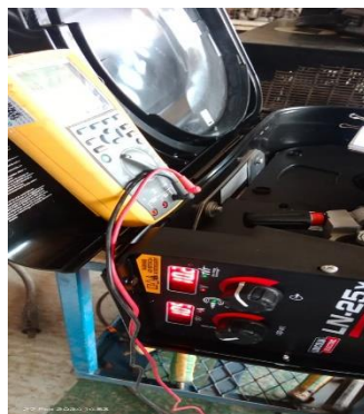
(a) Hasil Pengukuran constant current Welding equipment
