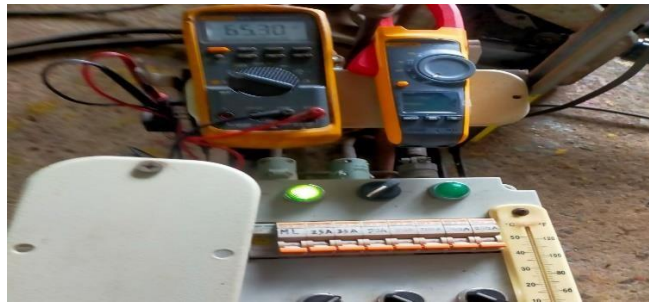
Gambar 7: Open Circuit Voltage
