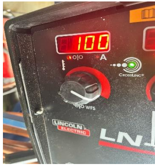
( c ) Hasil Pengukuran WFS Welding equipment
