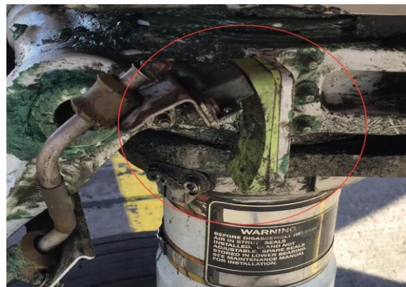
Gambar 2. Sensor corrosion /berkarat
