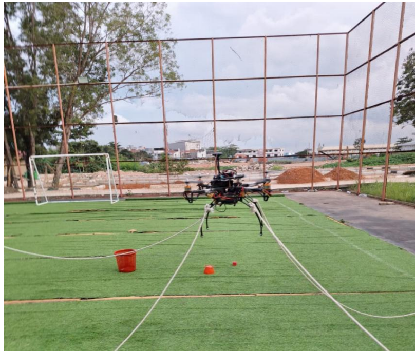
Figure 9. VTOL drone platform equipped with Raspberry Pi 5 during real-time outdoor testing under controlled tethered conditions.
