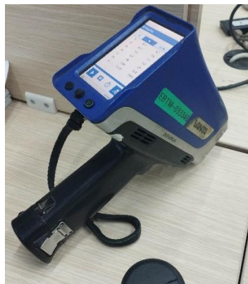
Gambar 2: PMI XRF portabel model VANTA
