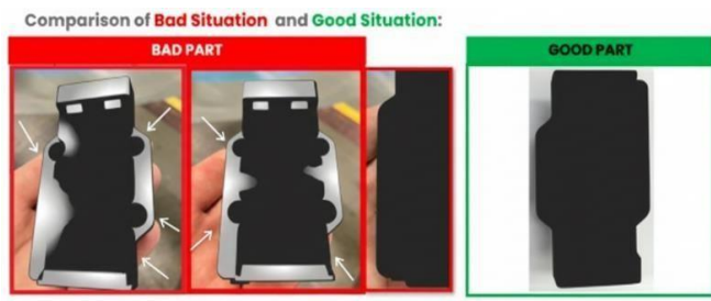
Figure 4. Comparison Bad Part and Good Part.
