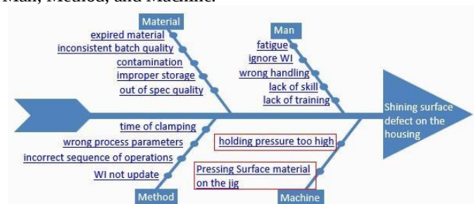
Figure 6. Ishikawa Diagram for Shining Surface Defect Cause Analysis.
