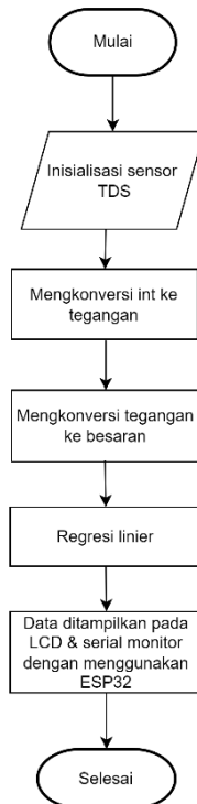
Gambar 11 Flowchart program sensor TDS
