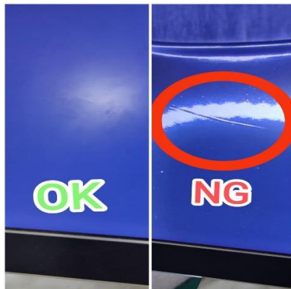
Gambar 3, Defect flow mark .
