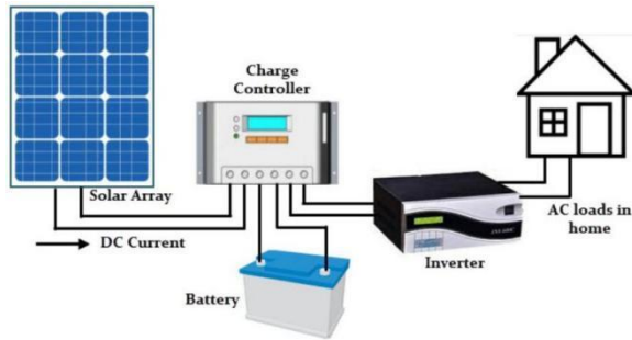
Gambar 7. Sistem PLTS Off-Grid
