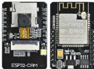
Gambar 3. Modul ESP-32 Cam
