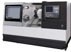
Gambar 5. Okuma Turning LB 4000 EX II
