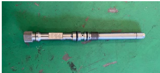
Gambar 18. Prechamber Valve Gas
