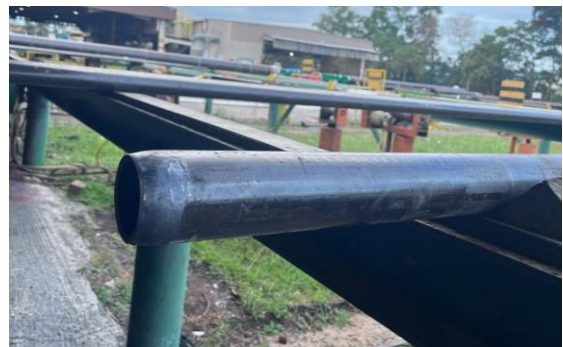
Figure 17. Pup Joints Size 2 7/8 Inch
