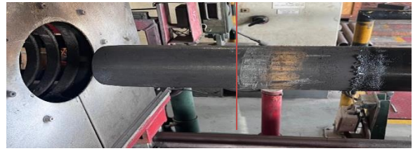
Figure 8. Material Pup Joint after combustion (Ok)
