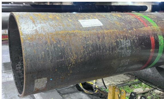
Figure 16. Pup Joints Size 16 Inch
