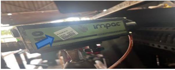
Figure 3. Sensor pyrometer not calibrate.
