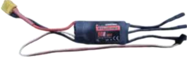
Fig 4. Hobbywing Skywalker 50a Ubec 5a Driver
