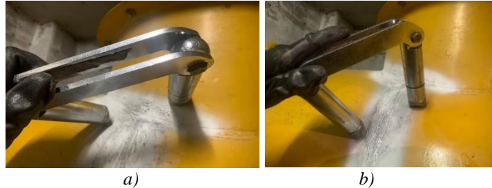
Gambar. 4 Pengujian Magnetic Particle Inspection a) head , b) shell
