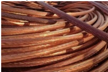
Gambar 13. Kabel Grounding BC
