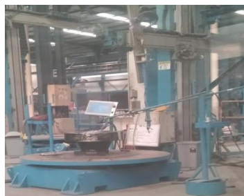
Gambar 6. Mesin Las GTAW ( Mechanized Welding )
