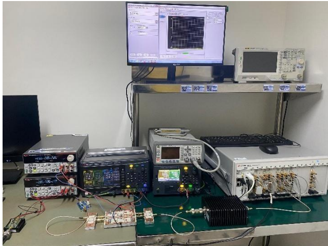
Figure 35: Measurement Parallel HPA Class-E Using VSG, VSA & Power Supply
