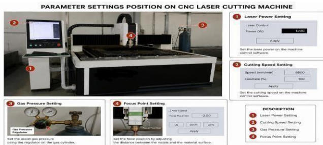
Figure 4 Parameter settings position on CNC laser cutting machine
