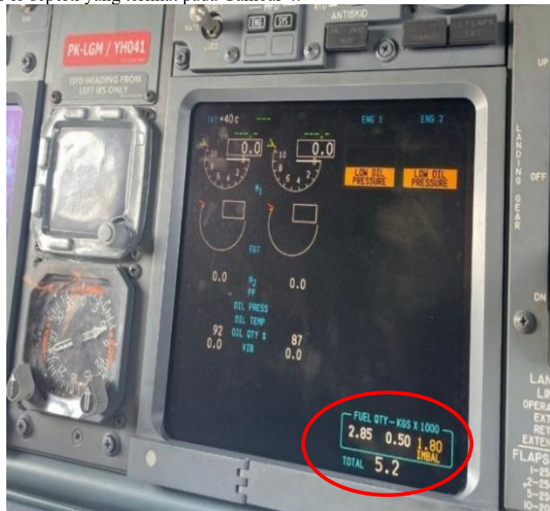
Gambar 4. Fuel imbalance in primary flight display
