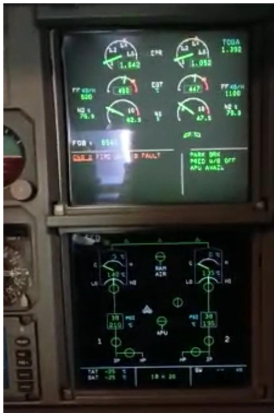
Gambar 11. Indikasi Bleed Precooler Temperature
