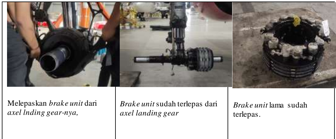
Gambar 10: Proses disassembly brake unit .
