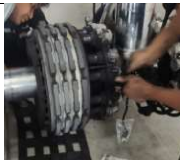
Melepaskan electrical connector dan hydraulic quick-release couplings .
