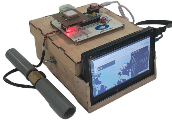
Figure 2. Prototype of the integrated navigation and fuel data acquisition module, consisting of an STM32-based sensor unit, GPS receiver, fuel flow sensor, and a Mini PC with a front-mounted display for web-based ship navigation simulation.
