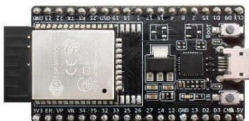
Gambar 4. ESP32 DevKitC V4
