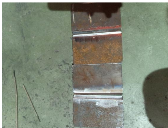
Gambar 3.2 Proses fit up single V butt joint
