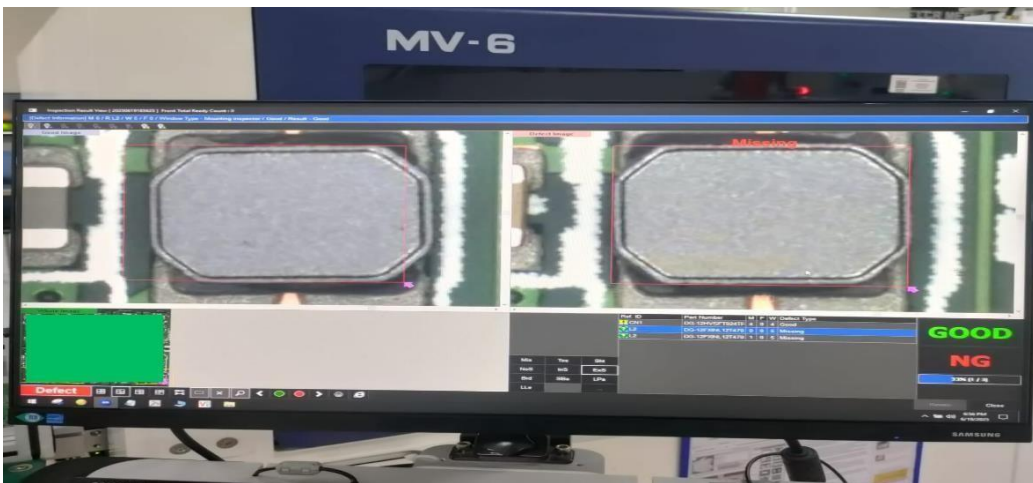
Figure 15. Defective display of SPI machine components
