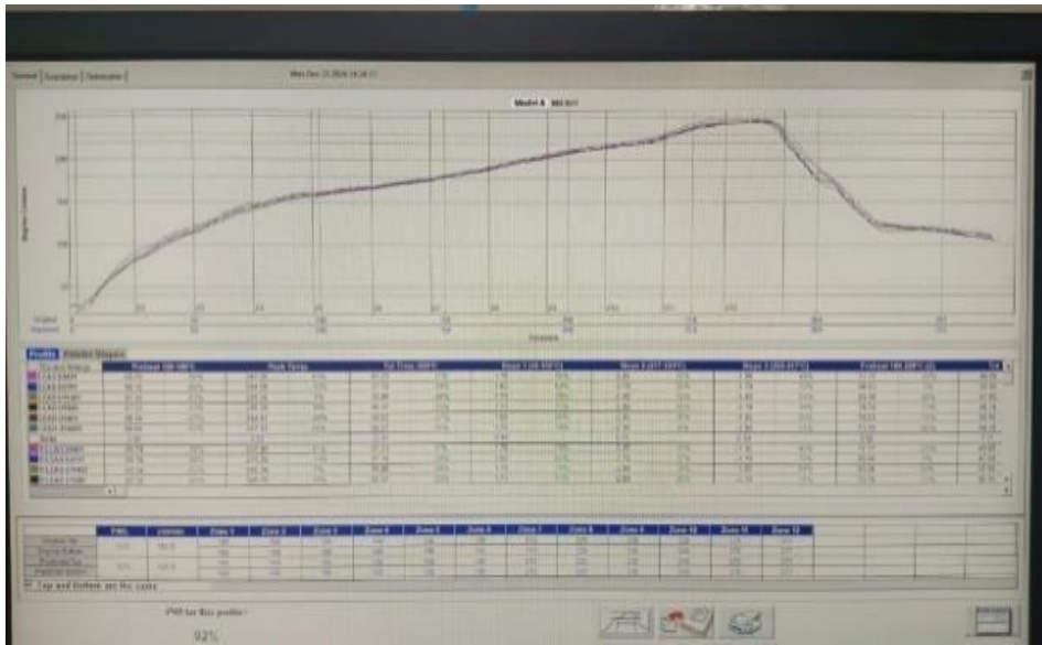
Figure 9. Display Reflow Temperature Profile
