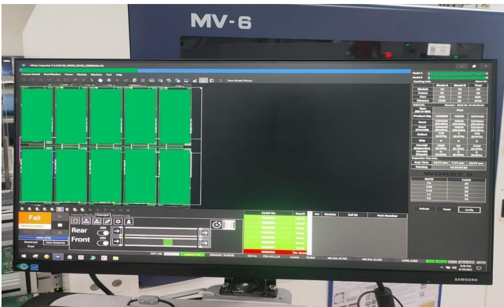
Figure 16. Defective display of SPI machine components
