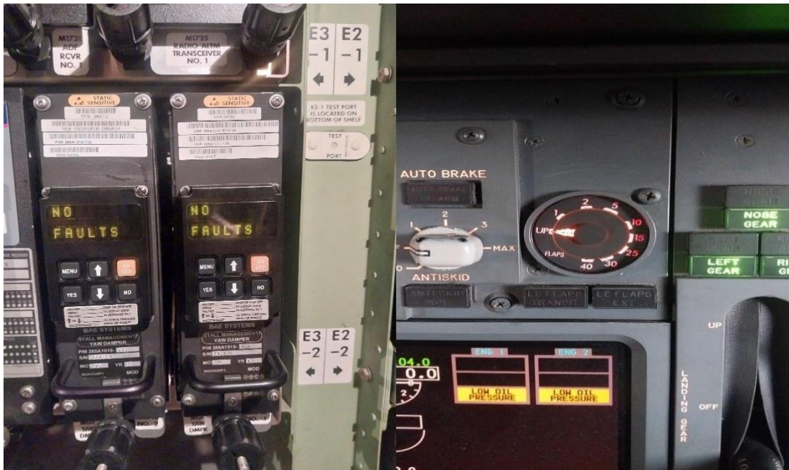
Gambar 4. Computer SMYD dan Position Indicator Flap.
