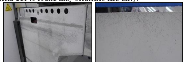
Figure 6. Dirty and scratches found on machine cover
