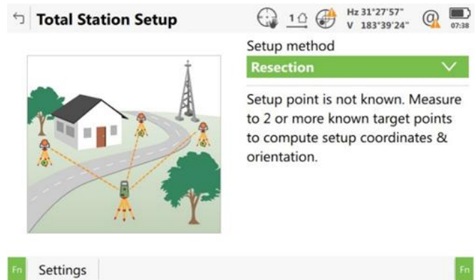
Gambar 6. Metode Resection (Sumber: Leica Total Station , 2023)
