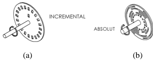
Figure 5 Example encoder types (a) Incremental encoder (b) Absolute encoder
