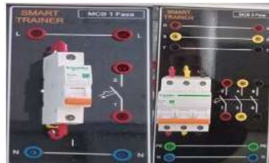
Figure 4.2. MCB Electrical Circuit Wiring
