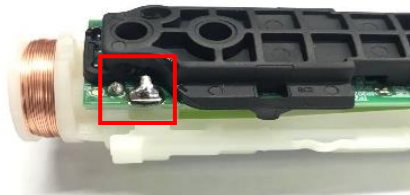
Gambar 6. Contoh Reject Solder Flag
