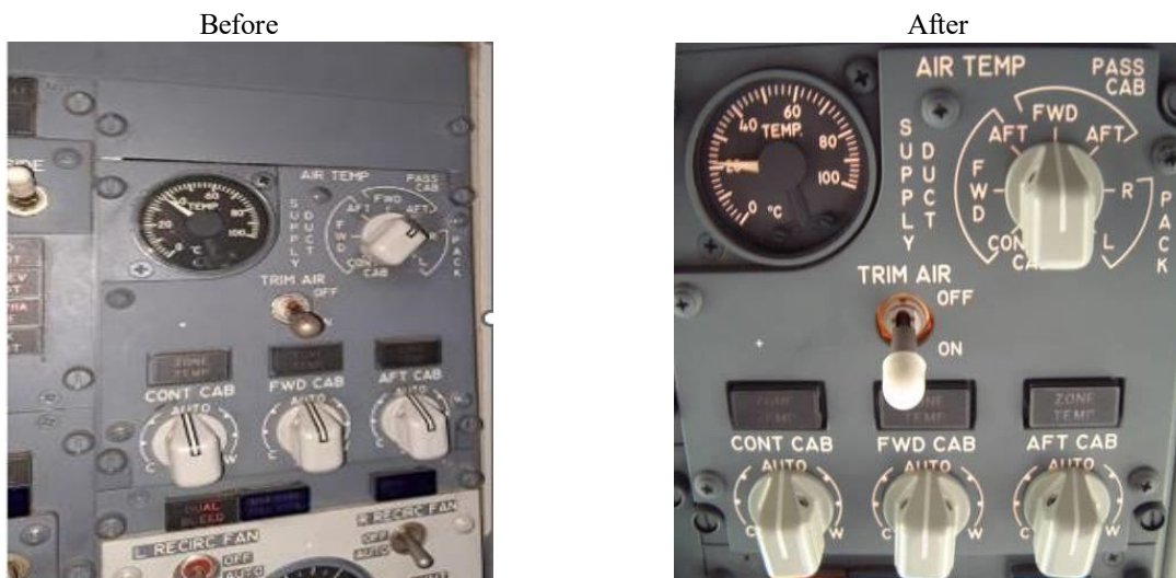
Gambar 6. Cabin Temperature Control [1]
