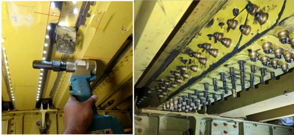
Gambar 12: Proses instalasi Upper Vent Stringer
