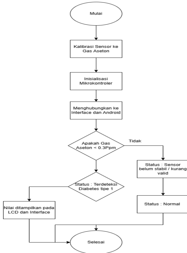
Gambar 8 Flowchart Sistem Alat
